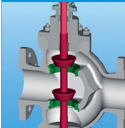
**Double seat with parabolic plug**
